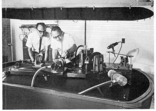
1000-POUND STEEL COVER is lowered when this rapid scan spectrometer is operated in a vacuum to permit rotating mirror (middle right) to reach 1100 revolutions/second. Physicist R. A. Hill (5122) adjusts a detector tube as engineer R. D. Fellerhoff (5141) looks on.
